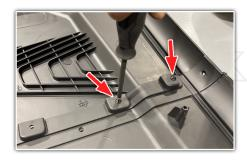
USE THE M6X20 SELF TAPPING SCREWS PROVIDED IN YOUR KIT TO FIX THE FRONT AND REAR PIECES OF THE ROOF TOGETHER AS SHOWN IN THE IMAGE TO THE LEFT.
