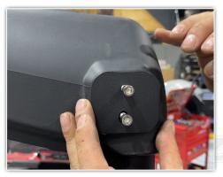
INSTALL THE RETAINER PLATES AT REAR CORNERS OF THE ROOF WITH THE M8X20MM FLANGE BOLTS.
