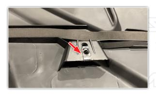
ATTACH THE THREE M6 THREADED CLIPS ONTO THE FRONT OF ROOF AS SHOWN.
