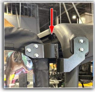
MOUNT THE DOOR: SLIDE DOOR ONTO PREVIOUSLY INSTALLED HINGE MOUNTS. BECAUSE EVERYTHING IS STILL LOOSE IT MAY BE NECESSARY TO WIGGLE THE DOOR A BIT TO GET IT TO SLIDE ALL THE WAY ONTO THE HINGE PINS. CLOSE AND LATCH THE DOOR GENTLY.
