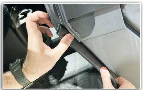
AFTER CLEANING MOUNTING SURFACE AND MAKING SURE THE GASKET IS ORIENTED CORRECTLY, PEEL BACKING FROM ADHESIVE A LITTLE AT A TIME AND GENTLY PRESS INTO PLACE EVERY FEW INCHES.
