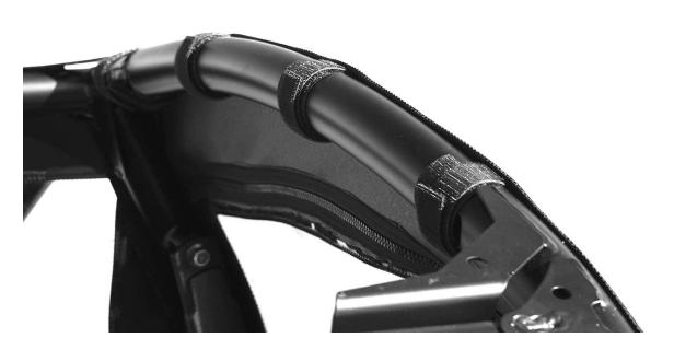
b. After installing the double-sided strips move to the rear of the door and attach the two Velcro tabs to the rear bar using the corresponding adhesive Velcro strip. See Photo Below:
