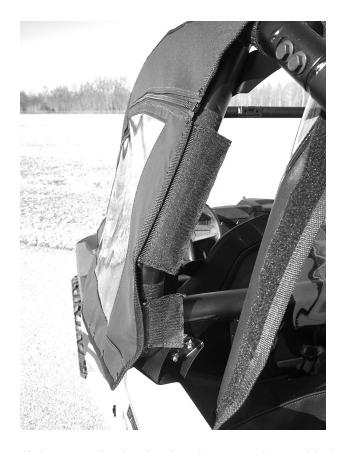
c. Next install the 12" adhesive hook strip to match up with the bottom of the front wing of the door as shown in the photo below.
