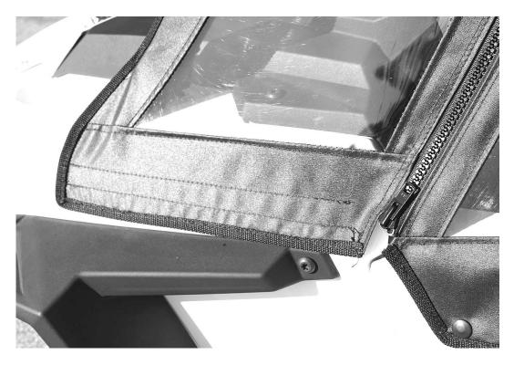
d. Lastly snap the bottom of the door to the plastic doors on the RZR. NOTE: it helps to place the screw snaps into the sockets on the cabs first, then starting at the top one, push them into the plastic so a small dimple is left behind. Then pull the screw snap back out and screw it into the plastic where the mark was made. See photo below:
