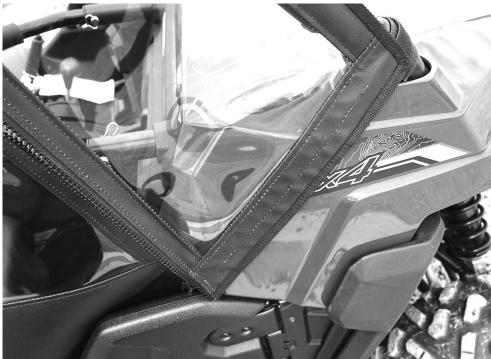
5. Once all the Velcro is in place the last thing to do is install the screw snap studs. Three go on the outside of the vehicle and one goes on the inside of the door.
