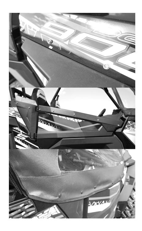
4. Lastly take the panels sewn to the inside of the doors and attach them to the door frames as shown in the photos below. The front panels have Velcro sewn to both sides to work with the door bags if you have them.
