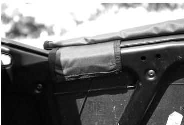
5. The larger panels on the inside of the doors are used to hold the doors in place after rolling them down as shown in the photo below. This helps keep the windows clean and free of scratches when rolled up.
