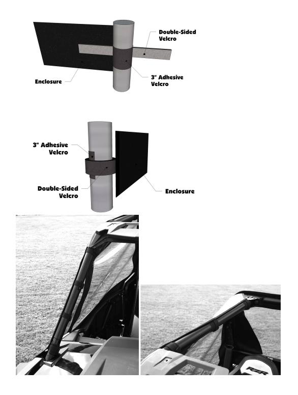
b. After installing the double-sided strips attach the 4" tab in the top front corner using the 4" adhesive strips. See Photos Below:
