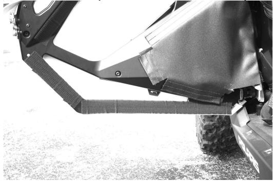
5. Finally place the door sweeps on the door as shown in the picture below.
