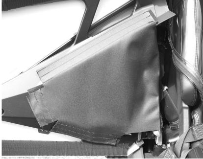
3. The next part is a little more difficult. Reach the back of the panel back between the seat and the back side panel while the door is wide open. You will notice where the is comes to. Take the 20" adhesive strip and place it there and attach the panel to it.
