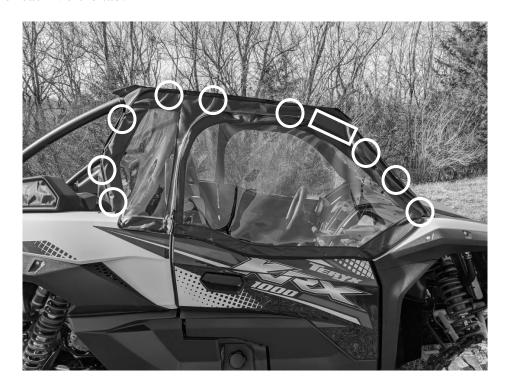
2. Next install the threaded snap studs into the body at the location of each snap. It is best to work from the front to the rear of the unit when installing the snap studs. The following image shows the location of each snap. Be sure to pull the door tight as you locate each snap stud to ensure proper fit of the door.
