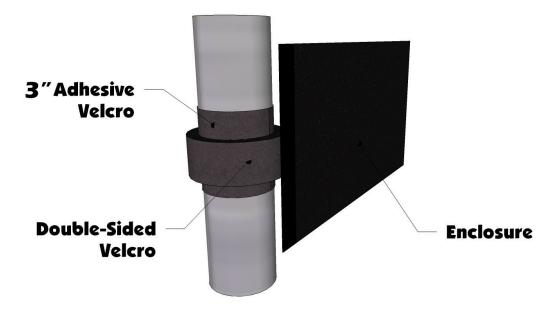
4. Next take the 20" adhesive Velcro strips and run it down the back of the roll cage facing towards the rear of the vehicle. Start at the bottom and work your way up the bar. You will see the double-sided Velcro tabs sewn along the back of the doors. See photo below.
