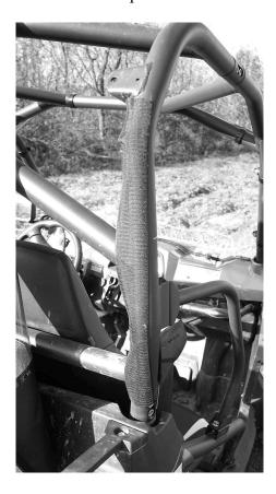
5. Once all the Velcro is in place the last thing to do is install the screw snap studs. NOTE: The best way to install the snap studs is to put them in the sockets in the door first. Then push them into the plastic to make a mark. Then pull the screw stud out and screw it into the plastic where the mark was made. See Photo on next page.
