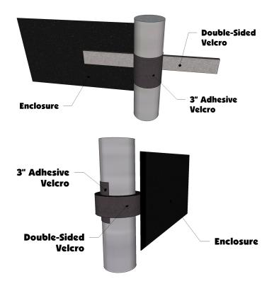
4. Begin installation of the Door Panels by hanging them from the Double-Sided Strips along the top of the doors. Hold the door up and mark where each strip is and wrap a 3" adhesive strip around the roll cage. Now hang the door up and it will be in place to install the rest of the Velcro for the door. See the photo below:
