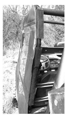
3. Once all the Velcro is in place the last thing to do is install the screw snap studs. NOTE: The best way to install the snap studs is to put them in the sockets in the door first. Then push them into the plastic to make a mark. Then pull the screw stud out and screw it into the plastic where the mark was made. See Photos Below.
