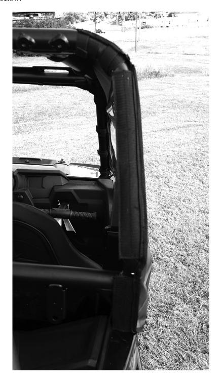
c. Lastly snap the bottom of the door to the plastic doors on the RZR. NOTE: it helps to place the screw snaps into the sockets on the cabs first, then starting at the top one, push them into the plastic so a small dimple is left behind. Then pull the screw snap back out and screw it into the plastic where the mark was made. See photo below:
