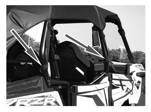
13. The last two straps attach to the end of the rear bars. Run the loop through the triangle hole where the two bars connect. See photo below:
