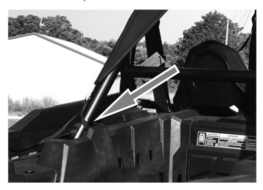
14. Finally make sure the top is centered and pull the straps tight. You may have to cut the ends of the straps and if you do make sure to melt the ends to prevent them from fraying out.
