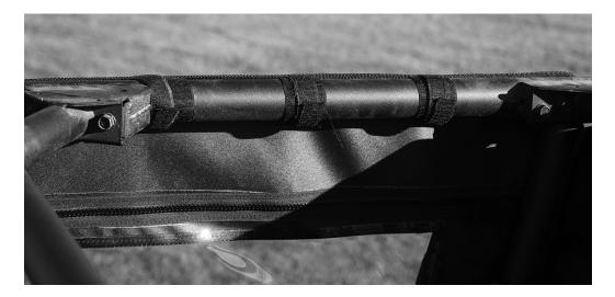
5. The rear edge of the front door also has double-sided strips as well but you do not use the 3" adhesive strips for it. Instead place the 45" adhesive strips down the backside of the middle bar facing the rear of the vehicle. You will need to cut the adhesive strip and place part of it above and below the mount for the bar as shown in the photo. See photo below.
