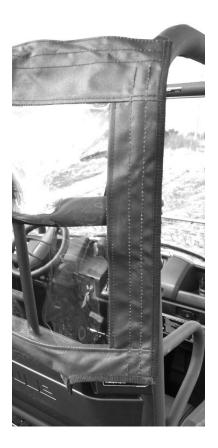
3. The bottom of the Rear Window is held in place by the 42" adhesive Velcro strip. The strip goes across the bottom on the plastic from one side to the other. The adhesive strips go on the bottom of the overhang on the plastic. The photos below show what it should look like.
