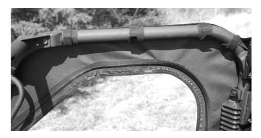
2. The rear edge of the doorshas a strip double-sided Velcro tab. Place the 17" adhesive hook strip down the rear of the roll cage. You will need to cut the Velcro so it adheres to each part of the frame.See photos below.
