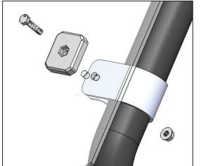
Adjust windshield as needed and tighten bolts.
