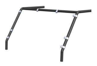
1. In the approximate locations shown, Snap 3 1.875" Plastic P Clamps on each side of the roll cage. The flanges will point forward and towards the center. Snap the smaller 1.75" clamps on the upper cross tube with the flanges forward and down.
