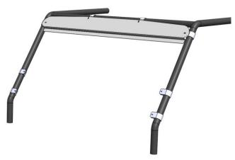
2. Holding the steel header panel in place with the flange facing IN, loosely bolt in place on each end using the M6X20 flange bolts and nyloc nuts as shown in step 3.
