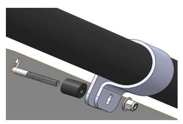
**4.** Bolt the header panel loosely to the upper crossbar using the M6x45 flange bolts, plastic spacers and nuts. Leave all header panel fasteners slightly loose so you can adjust its position after the windshield is in place.
