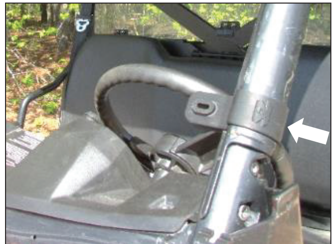
12. Attach the pro-fit roll cage clamps to the vehicle in the approximate location shown.
