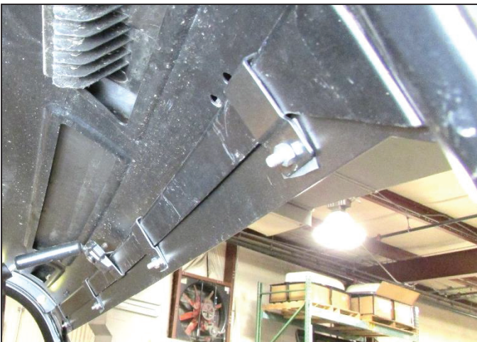
11. Flip the header panel brackets over and attach secure to the vehicle by tightening the hardware. See step 9 for details.
