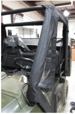
1. Mount side panel cab sections positioned correctly & taught. NOTE: You will cut the side panels - Ensure they are positioned correctly.
