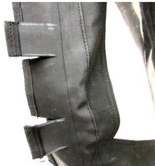
4. Cut fabric across. Do not cut past the first vertical seam
