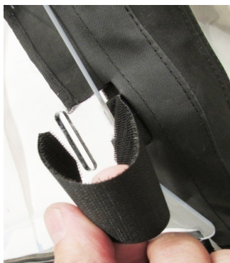
7. Install straps lacing through the flap opening to the inside of the cab and secure velcro
