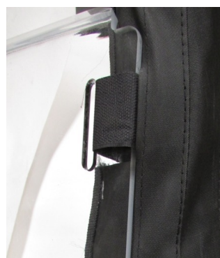
7. Install straps lacing through the flap opening to the inside of the cab and secure velcro
