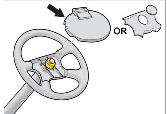
3. Remove the nut and steering wheel from the shaft. Retain hardware and steering wheel for reinstallation.
