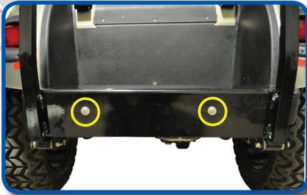
Attach bagwell bracket to rear of cart as shown using hardware from pack 2.
