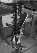
5) Next, insert the spring stiffener onto the shock.
