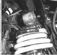
4) Using a spring compressor, compress the shock and remove the stock spring.
