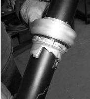
6) Place the stock spring(s) back onto the shock.
