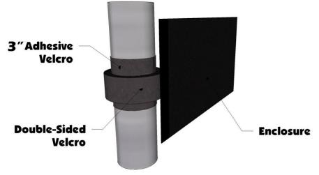
5. After attaching the double-sided strips go to the rear of the door. You will see three Velcro tabs sewn here. Starting just below the top cross bar place the 32" adhesive strips down the bar facing the rear of the vehicle. Then pull the tabs around and attach then down the bar to the Velcro. See Photos below.
