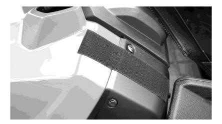
7. Last Item on the doors will be a snap on the inside front section of the plastic doors. Its easier to place the snap in the right position by first putting the screw snap stud into the socket on the enclosure. Then pull the door into place and push the snap into the plastic so that an mark is left. Then pull the snap out and screw it into the door making sure not to over tighten and strip out the plastic. See Photos Below.
