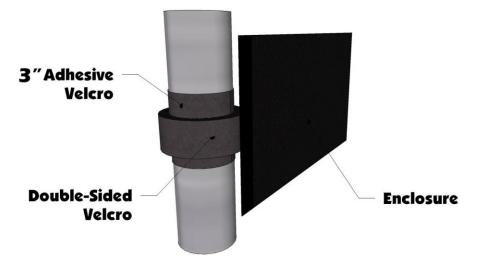
**5.** After attaching the double-sided strips go to the rear of the door. You will see three Velcro tabs sewn here. Starting just below the top cross bar place the 32" adhesive strips down the bar facing the rear of the vehicle. Then pull the tabs around and attach then down the bar to the Velcro. See Photos below.
