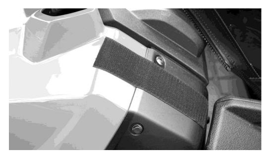
7. Last Item on the doors will be a snap on the inside front section of the plastic doors. Its easier to place the snap in the right position by first putting the screw snap stud into the socket on the enclosure. Then pull the door into place and push the snap into the plastic so that an mark is left. Then pull the snap out and screw it into the door making sure not to over tighten and strip out the plastic. See the following photos.
