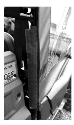
**6.** Now move to the front lower corner and place the 9" adhesive strip to match up with the Velcro on the cab. See Photo Below.
