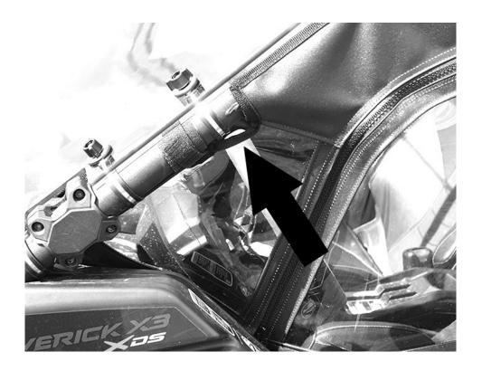
7. The rear of the door has two double-sided Velcro strips that attach to the main bar towards the rear and the short downward bar as shown in the photo below
