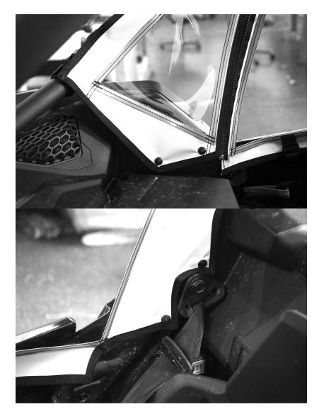
9. Lastly take the 3 straps along the bottom of the door and attach them to the main door frame as shown in the photos below.
