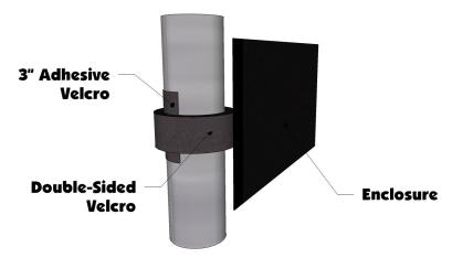
4. Begin installation of the Door Panels by hanging them from the Double-Sided Strips along the top of the doors. Hold the door up and mark where the each strip is and wrap a 3" adhesive strip around the roll cage. Now hang the door up and it will be in place to install the rest of the Velcro for the door. See the photo below:
